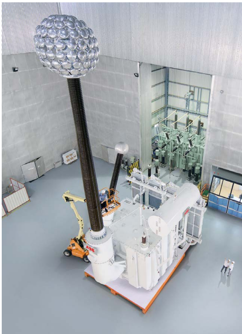
Figure 5. ABB's 1,200 kV AC transformer was developed, manufactured and tested at ABB's Vadodra facility in India and currently supports India's central transmission utility, at Bina India.
